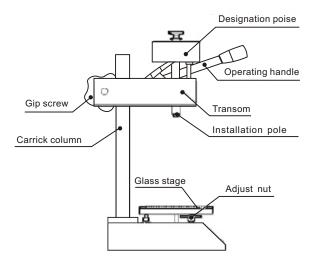
The Test Stand construction include operating handle, regulable glass stage, designation poise, transom, Gip screw, and carrick column. After adjustment the value will be more accurately.
